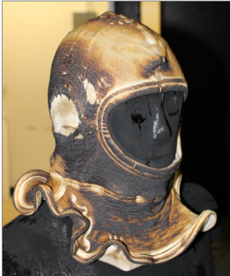
Traditional Hood - 100% meta-aramid 7-second flashfire exposure Hood-only configuration
