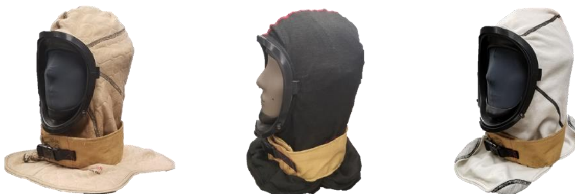
Figure 11: System-Level Thermal Sweating Head for Heat Loss
