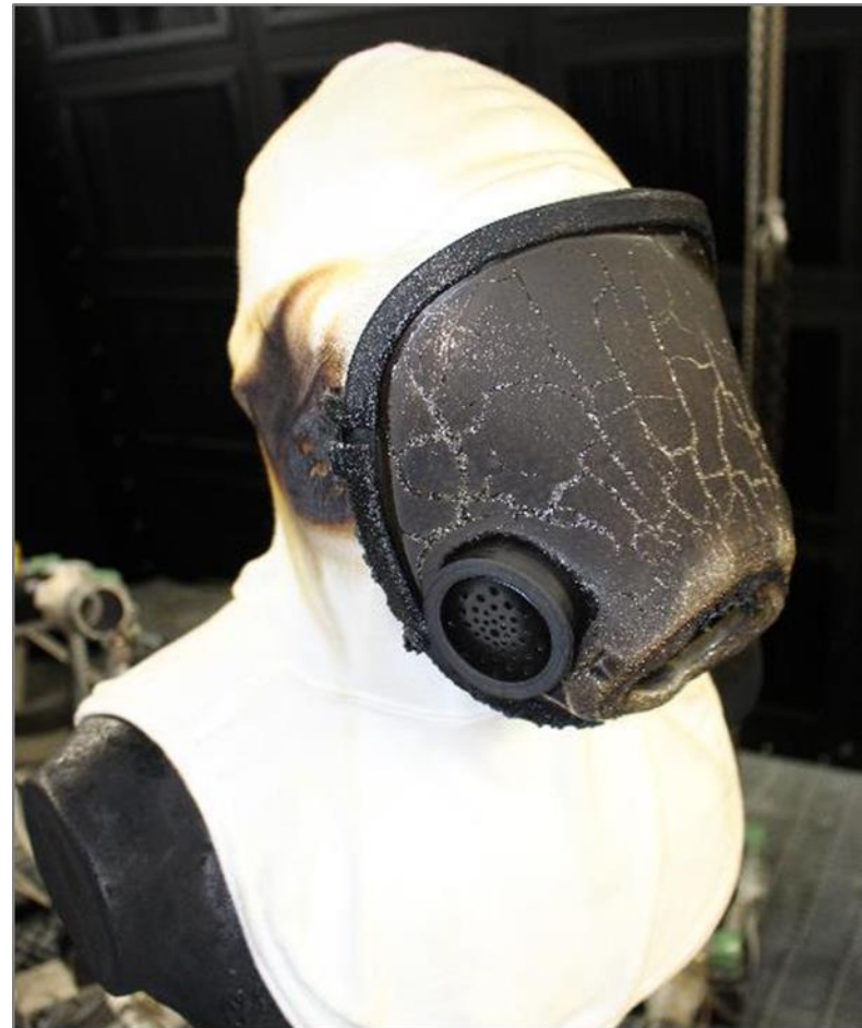
Traditional Hood - 100% meta-aramid 12-second flashfire exposure Full head ensemble configuration (hood, mask, helmet, ear flaps, jacket)
